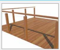
Pass the opposite end of the wire through the pre-drilled intermediate posts.
