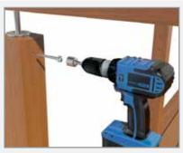
Use the socket head drive bit to drive the screw eyes into the pre-drilled end posts. **Note:** The screw eye should be driven into the post so as only the head of the screw eye is visible.
