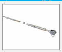
Remove the rigging screw and nut from the opposite end of your wire, this will allow you to pass your wires through the pre-drilled 7.5mm holes in your intermediate posts.
